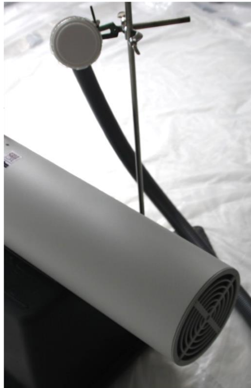
Figure 10: Illustration of the experimental setup and representation of the positioning of the gelatin filter respectively of the B AIR V2 system.
