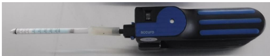
Figure 8: Dräger pump with test tube for ozone measurement.
