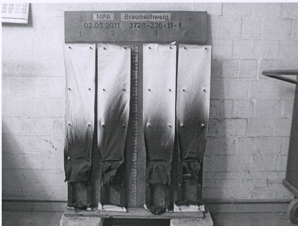
View of the specimens (cotton fabric with weight per unit area of 137 g/m 2 , with "KAPPAFLAM CFP" fire retardant) after the "Brandschacht" reaction to fire test
